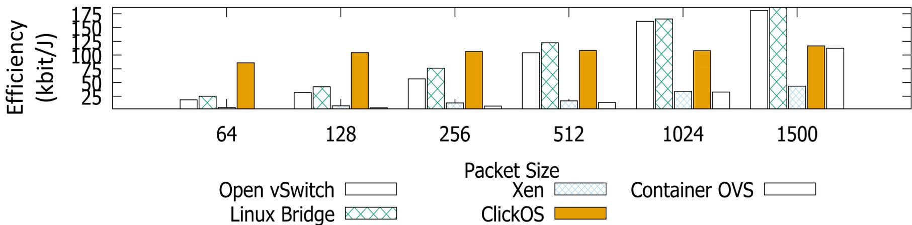
Energy efficiency of packet forwarding in various NFV installations
